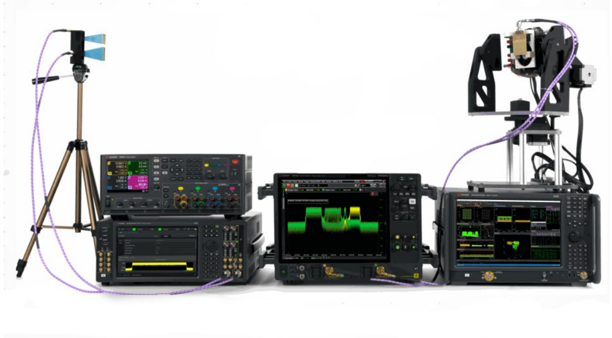
Figure 2. 5G NR 28 GHz MIMO test setup
