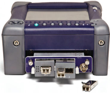
Scalable, modular design with pluggable physical interface (PIMs) and small form-factor (SFPs/XFPs) modules
