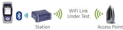
OneExpert controls the Wifi Advisor for Single Ended Operation with Best Channel
