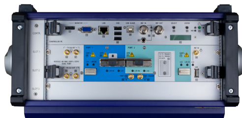
Dual-port CFP2 plugged into ONT-603 Mainframe
