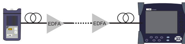
PMD test configuration through amplified link
