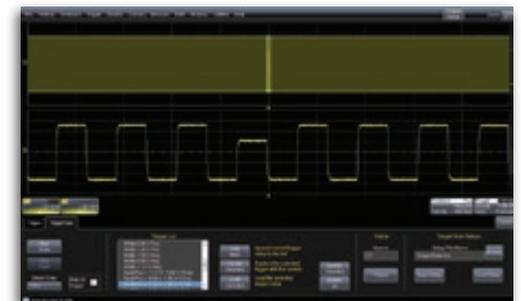
A 1 in a billion rare event seems fast but is only 5 seconds of circuit operation on a 200 MHz clock. TriggerScan finds the rare event in 4 minutes while an oscilloscope with 400,000 waveforms/second capture rate misses 99.8% of the signals and could spend nearly 42 minutes to find the error.
