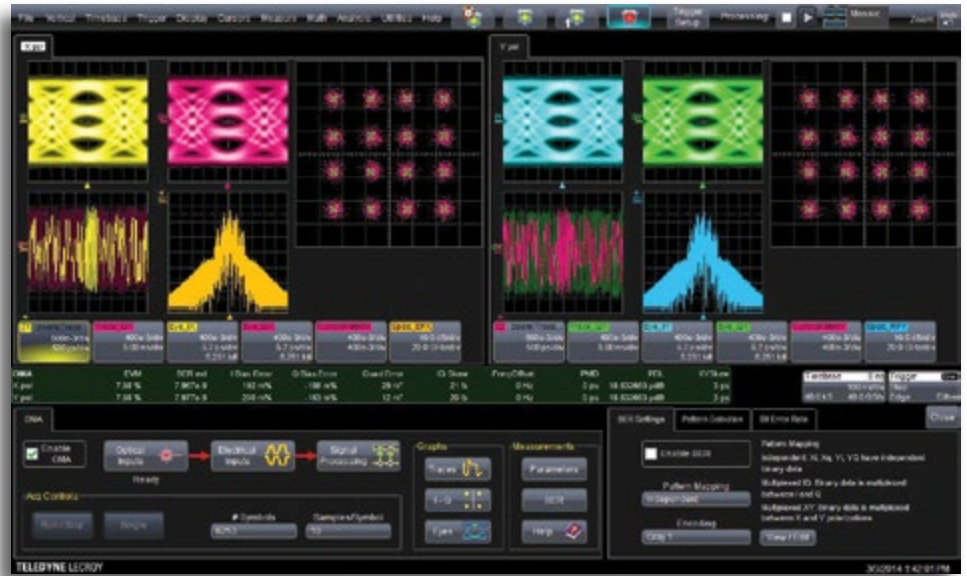
Analysis of a DP-QPSK optical signal.
