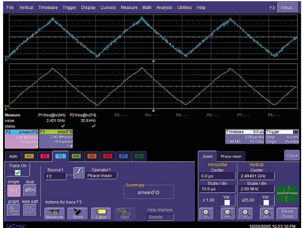
See multiple cycles of spread spectrum clocking.
