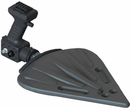
Alaris direction-finding smart antenna.
