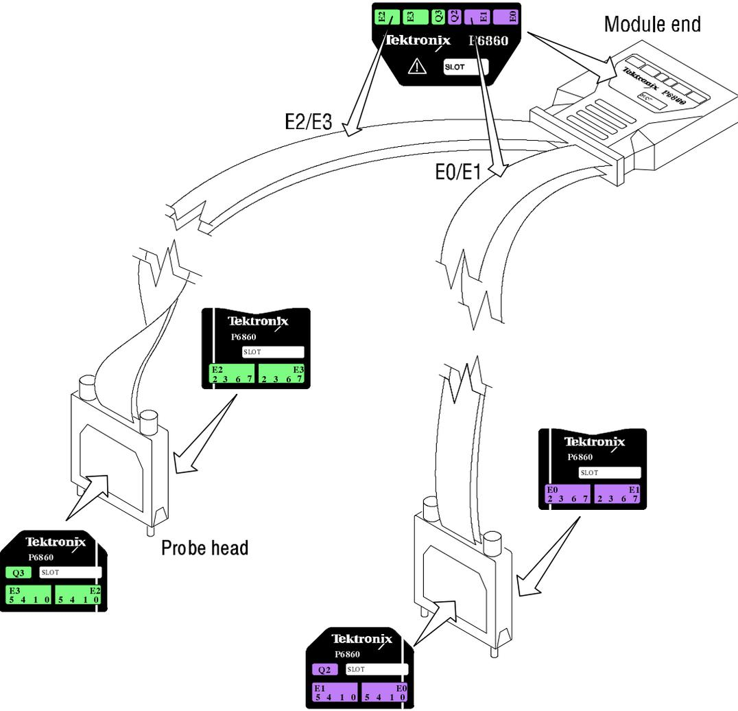
Figure 2: Attaching the P6860 High Density probe labels
