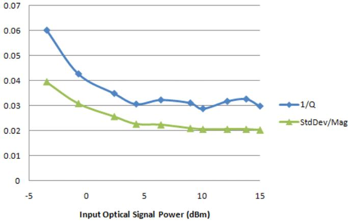
Figure 7 – Constellation diagram accuracy including intradyne and demodulation error can be measured by the RMS error of the constellation points divided by the magnitude of the electric field for each polarization signal. The following data has been measured on a 2.5 Gbaud NRZ 1-pol QPSK transmitter using a Tektronix MSO72004 digitizer.
