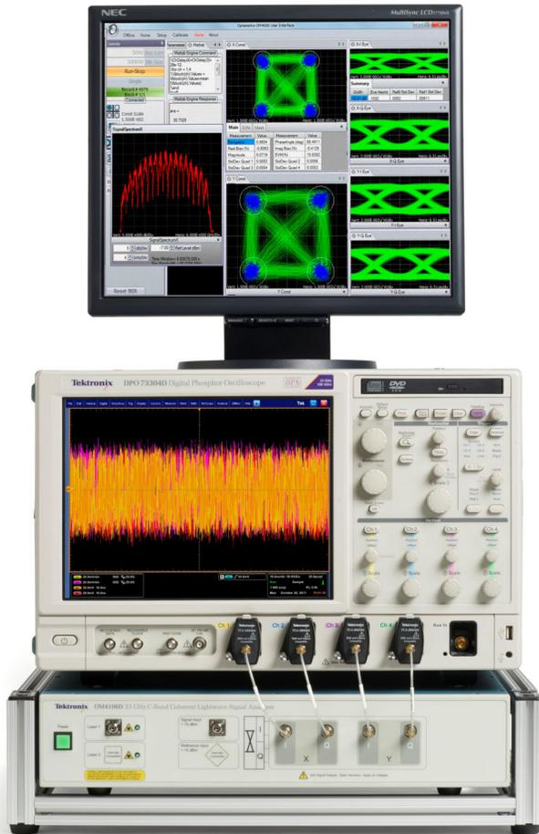
OM4000 Series Coherent Lightwave Signal Analyzer and Tektronix DPO70000 Series Oscilloscope.
