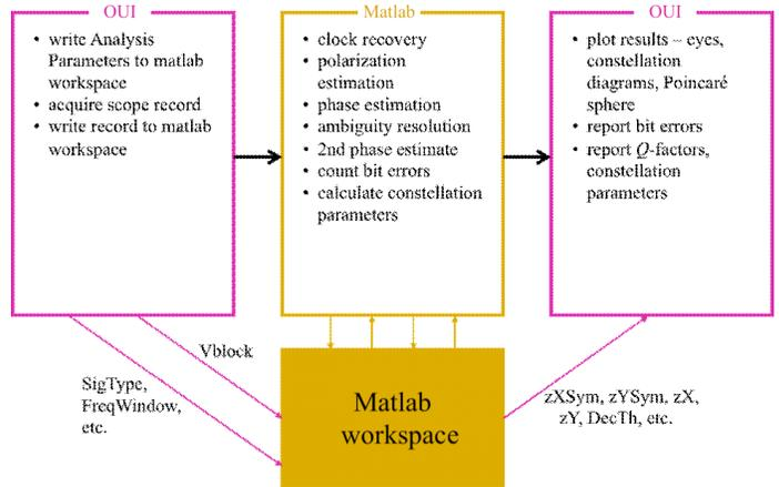
Figure 3 – Illustration of data flow under control of the OUI.
