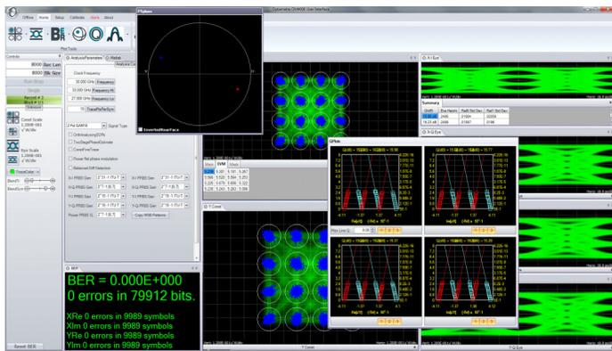
Figure 5 – QAM Measurements on the OM4000 User Interface (OUI).
