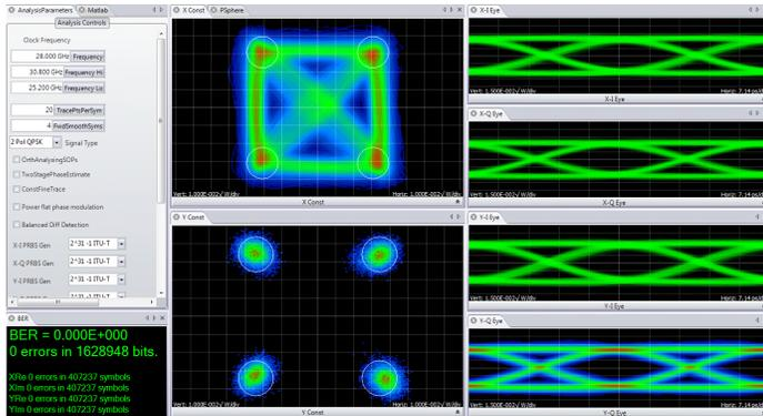
Figure 1 – OM4000 User Interface (OUI) showing color-grade graphics options. Symbols can also be colored to a key indicating prior state. Data shown is 112 Gb/s PM-QPSK.
