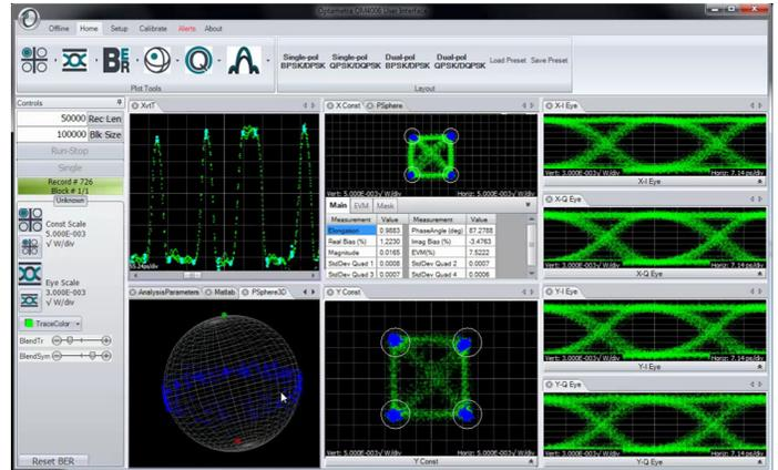
Figure 2 – OM4000 User Interface (OUI) showing display of select equivalent-time measurements.
