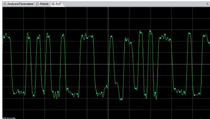
Errored symbol in Measurement vs. Time plot.
