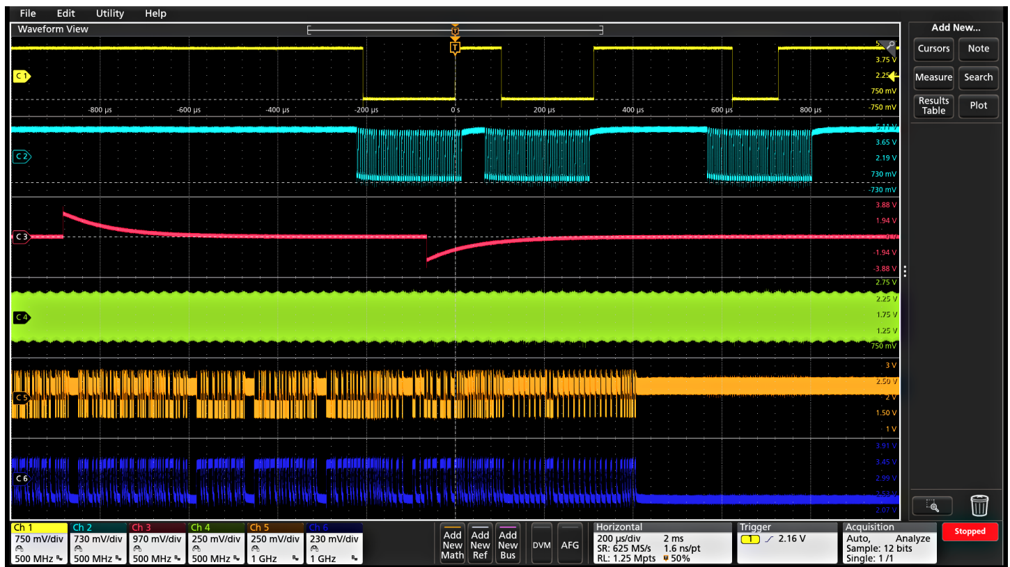
Using multiple channels to visualize multiple clock and data lines.
