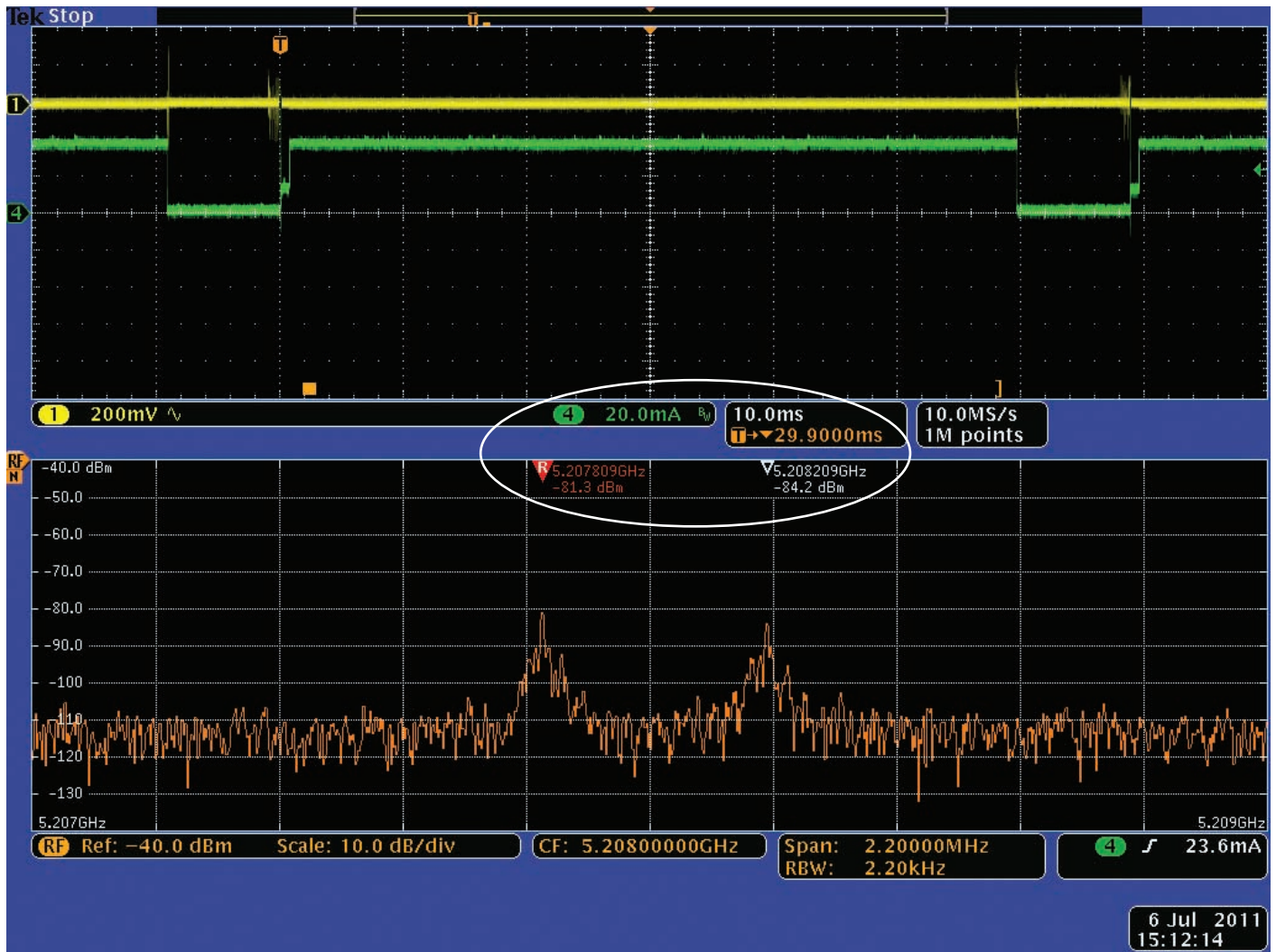
Figure 13. Spectrum at the sixth harmonic. Peak values of markers show signals down -80 dBm.
