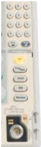
Figure 5. User controls for MDO Frequency Domain Display.
