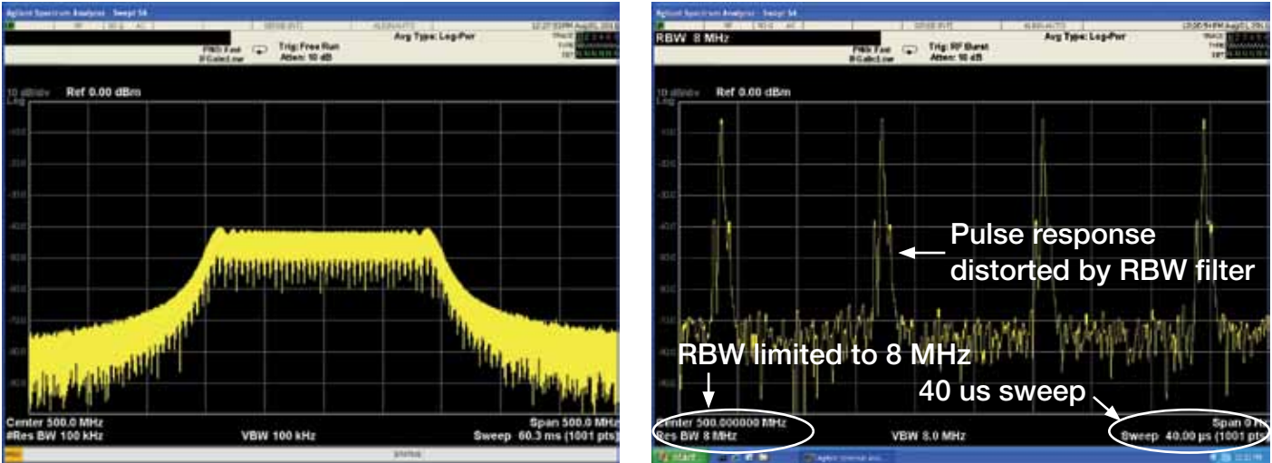
Figure 9a/9b. Shows a wideband pulse signal in spectrum (a) and zero span (b) time domain view.
