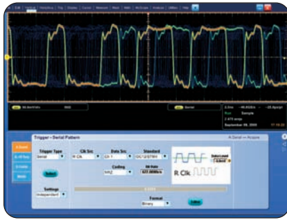
► Serial pattern triggering to debug pattern-dependent issues.
