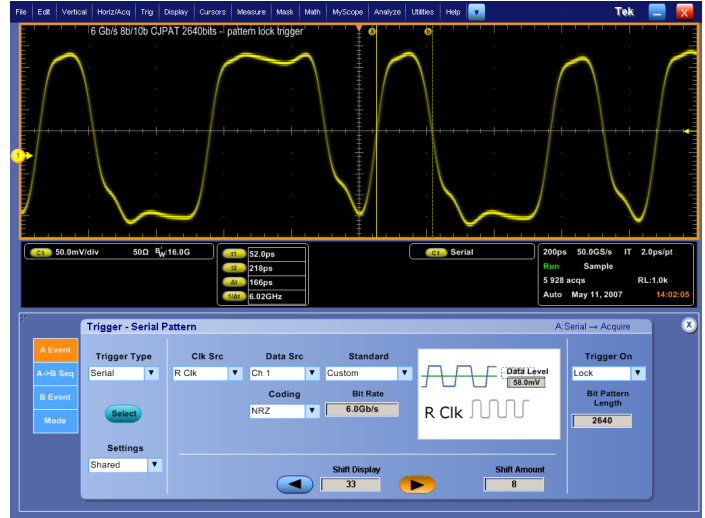
NRZ Pattern Lock Triggering of a 640-bit long SATA serial pattern at 6 Gbps
