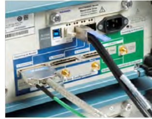
UltraSync connection on instrument with Master role
