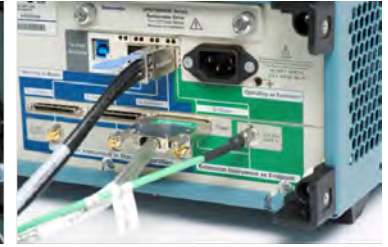
UltraSync connection on instrument with Extension role
