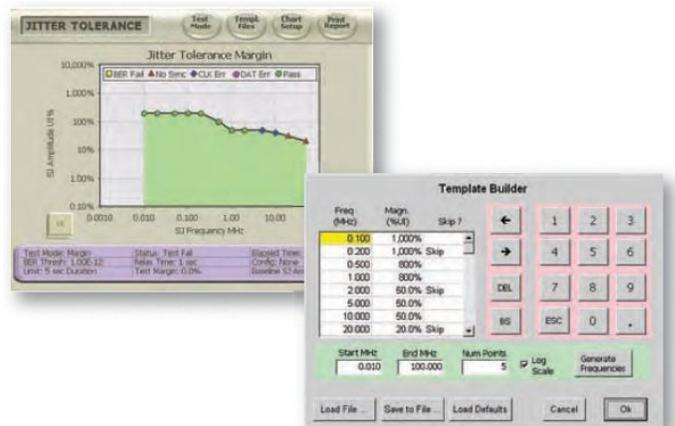
Built-in jitter tolerance function
