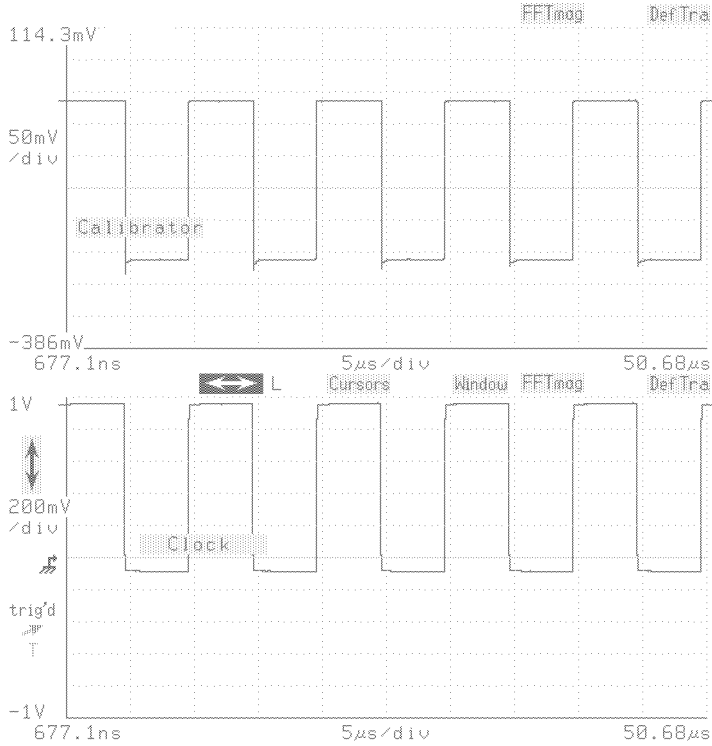
Figure 2-19: A Dual-Graticule Display
