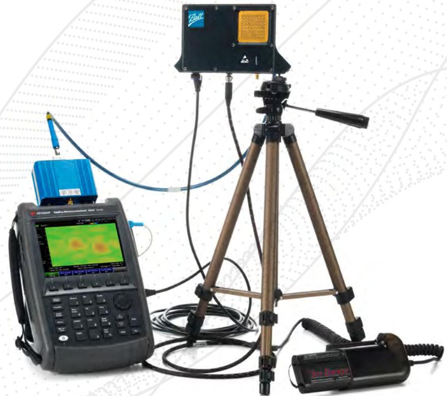
Figure 2. FieldFox and phased array antenna set up
