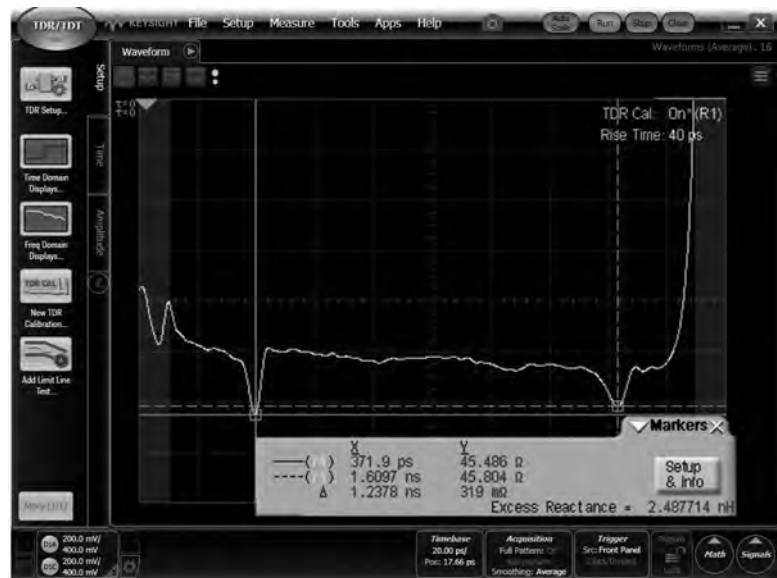
Figure 1.10: TDR Response from a Microstrip with Two Reference Pads Using Markers to Measure the Round-Trip Time Delay
