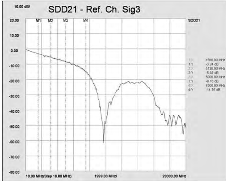
Figure 6.30: Reference Channel Insertion-Loss
