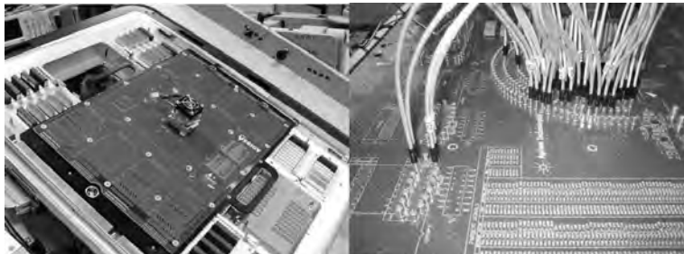
Figure 19.2: Example of an ATE Test Fixture for Multi-Gigabit Graphics Device (Left), Using Coaxial Cables to Try to Avoid the PCB Signal Trace Loss (Right)
