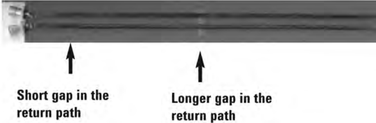
Figure 1.43: Tightly Coupled Pair of Transmission Lines with Small Gaps in the Return Path That Will Generate Ground Bounce
