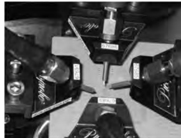
Step 2: Attach Microprobes to the Ends of the VNA Cables. Step 3: Perform All the Measurements with Microprobes
