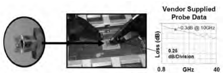
Figure 10.2: The GGB Picoprobe GSG with 400 um Pitch (Left), Probing an ATE Test Fixture (Middle) and Insertion Loss Performance of the Probe Measured by the Manufacturer (Right)
