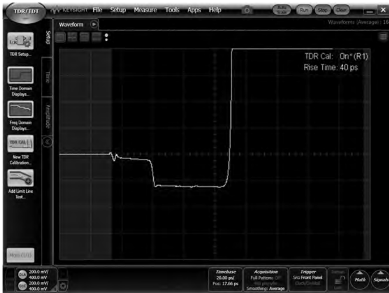
Figure 1.4: The Same Transmission Line Displayed on the Impedance Scale at 10 Ohms/div, with 50 Ohms in the Center
