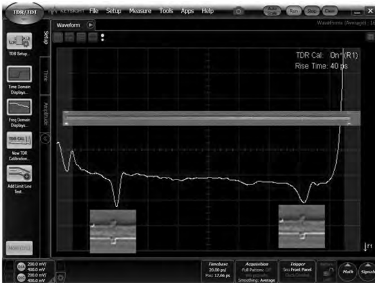
Figure 1.9: TDR Response of a Uniform Transmission Line with Two Small Reference Pads Located on Four-Inch Centers
