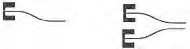
Figure 22.13: The new 1-port AFR method in PLTS 2013 doesn't require any calibration standards to be fabricated. The fixture to be removed is simply measured with an open circuit at the reference plane.
