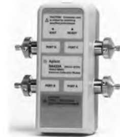
Figure 8.20: Steps for Using De-Embedding in Calibration. Step 1: Calibrate All Ports at the End of the Coax Cable Using the Electronic Calibration Module
