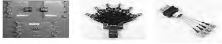
Figure 22.7: Most standard interface test fixtures have a coaxial connector interface (SMA, SMP, 3.5 mm, 2.4 mm, etc) at one end to connect to the test equipment
