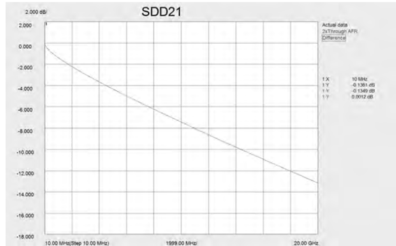
Figure 23.9: Actual data vs 2XTHRU AFR
