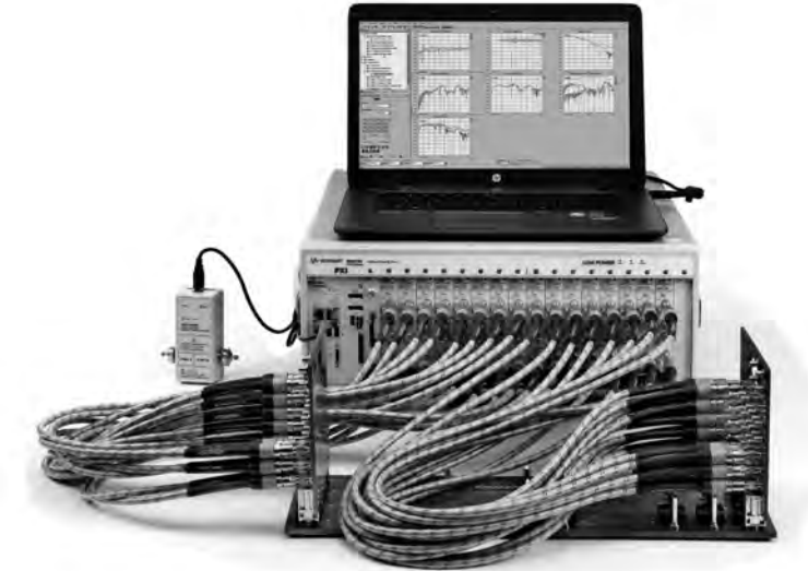
Figure 5.4: Typical multi-port Vector Network Analyzer from Keysight Technologies that can handle up to 32-ports. Reference part numbers are as follows: M9375A PXI VNA, N1930B PLTS software and N4691B Opt. 00F ECal.
