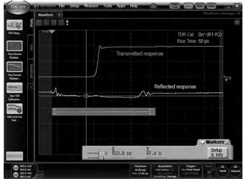
Figure 1.29: Example of TDR/TDT Response from Eight-Inch-Long Microstrip Transmission Line on 20 mV/div and 500 ps/div Scales
