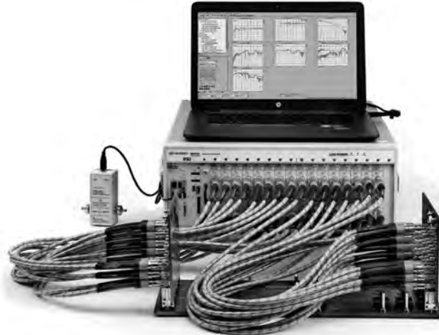
Figure 6.10: The standardized PXIe chassis is a typical platform for a multi-port vector network analyzer test system using Physical Layer Test System (PLTS) software. Up to 32 ports can be supported today
