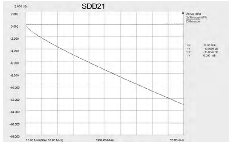
Figure 23.12: Actual data vs 2XTHRU AFR
