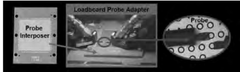
Figure 10.3: Example of an Interposer Designed for a Specific BGA Ball-Out (Left), Interposer Attached to the Loadboard for Probing Connection (Middle), and 400 \mu m G-S-G Probe Tip Connection to the Probe Interposer Board (Right)
