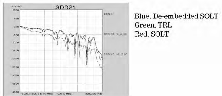
Figure 12.19: Applying Correct Dielectric Constant of PCB Material Shows Correlation between De-Embedded SOLT and TRL
