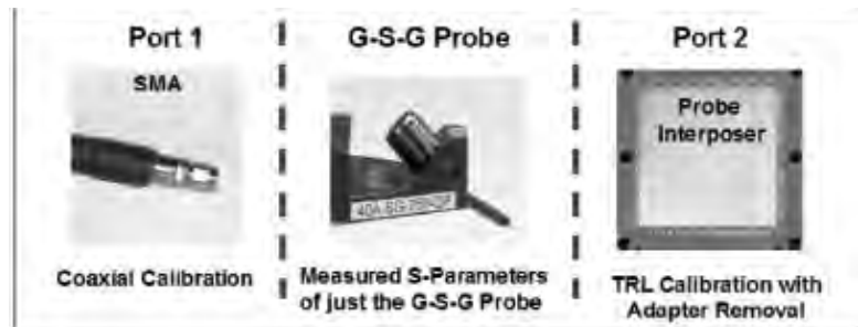
Figure 10.7: Utilization of TRL Calibration Standards and Adapter Removal Methods to Move the Measurement Plane to Either Side of the G-S-G Probe so That the Electrical Performance Can Be Measured for the Desired Application
