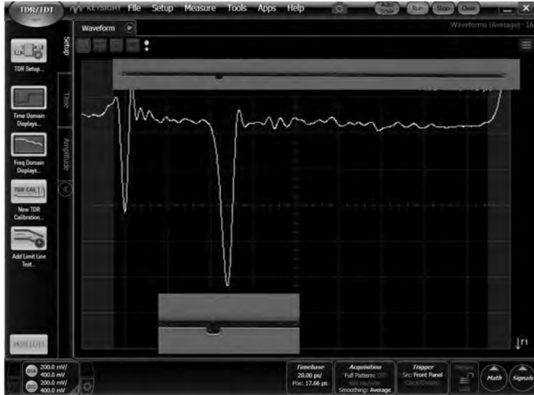
Figure 1.14: TDR Response from a Uniform Transmission Line Having a Small Test Pad
