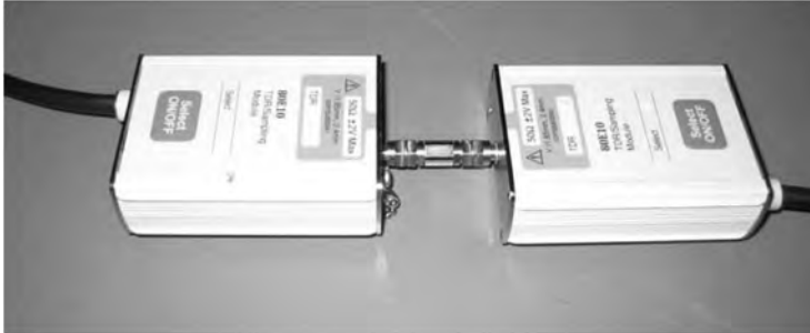
Figure 11.3: Photo of the Transmit and Receive Channel of One Line in a Pair, Connected in a Thru Reference Configuration
