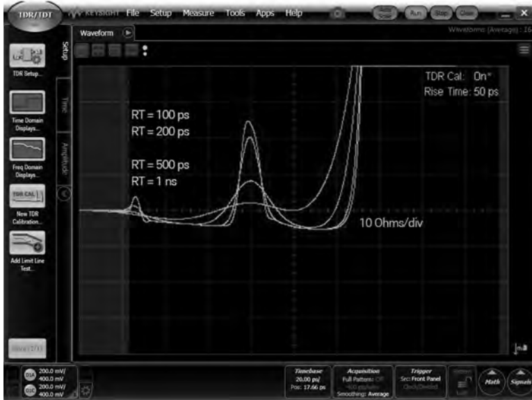
Figure 1.61: Emulating the Differential Impedance Profile of a Differential Signal Crossing a Large Gap at Four Rise Times
