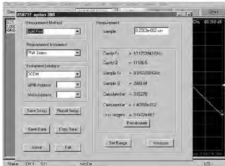
Figure 16.10: User Interface Screen for Entering Sample Thickness and Initiating the Measurement
