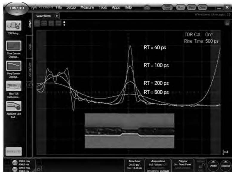
Figure 1.26: Emulating System Rise Time Responses for a 200 mil Long Neck Down Region with RT = 40, 100, 200, and 500 ps
