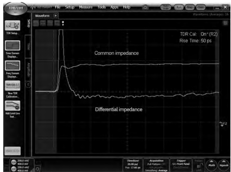
Figure 1.59: Measured Reflected Common Signal from a Coax to Twisted Pair Transition with an Incident Common Signal
