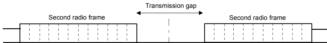
Fig. 4-26 Envelope of compressed mode signal with double-frame method
