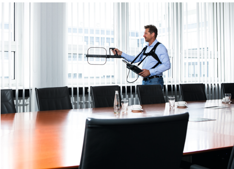
Finding bugs with the R&S®PR100 and the R&S®HE400 active directional antenna.
