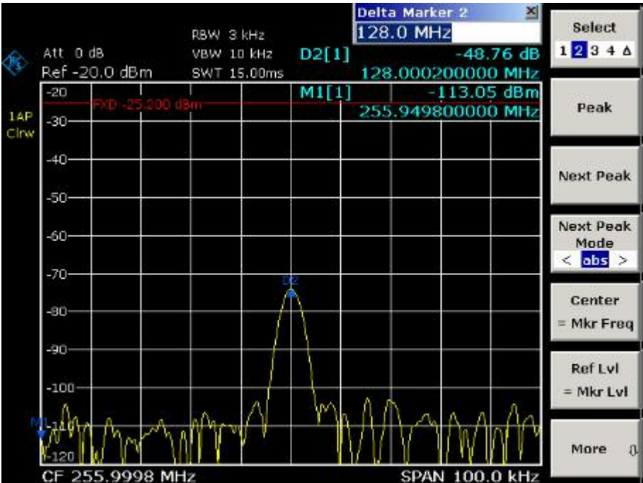
Fig. 2-3 Measuring the level difference between the fundamental wave (= reference point level) and the 2 nd harmonic
