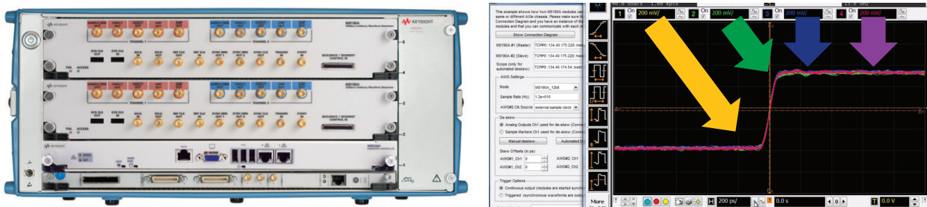
Figure 18. The Keysight M8190A 12 Gsa/s is a high-resolution AWG with up to 14 bits of resolution that can support up to 12 synchronous channels with sub nanosecond time adjustments, which are important capabilities in multi-channel test scenarios. Shown here are four channels synchronized to such levels on a four-channel oscilloscope.
