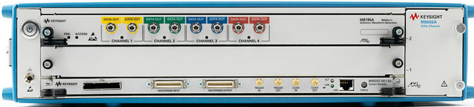
Figure 17. The M8195A is a high performance, 8-Bit Arbitrary Waveform Generator with sample rates of up to 65 GHz and an analog bandwidth of 20 GHz.
