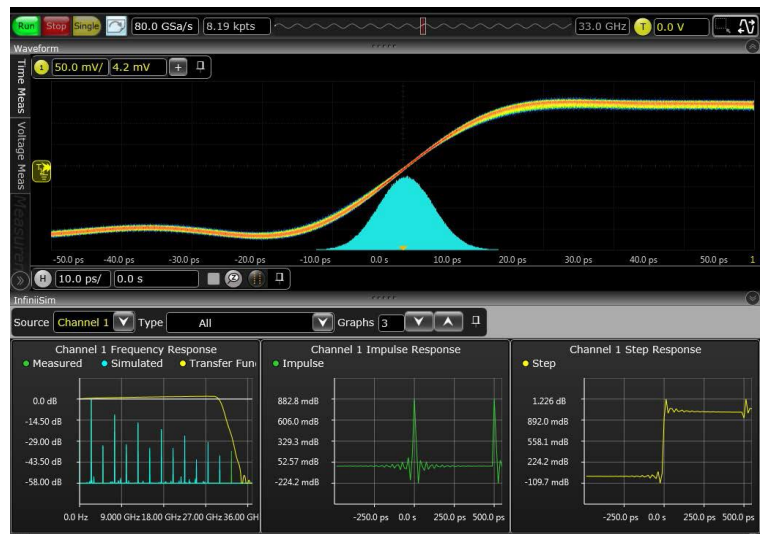
InfiniiSim renders the waveform through hardware acceleration
