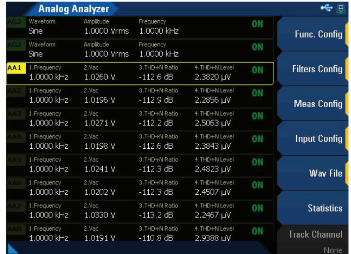
Figure 4. The U8903B's GUI, showing 8 analyzer channel measurements.
