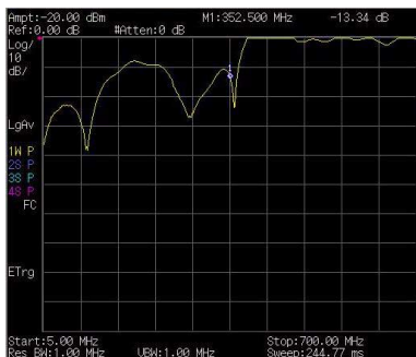
Figure 3-22 Measuring the Return Loss of the Filter
