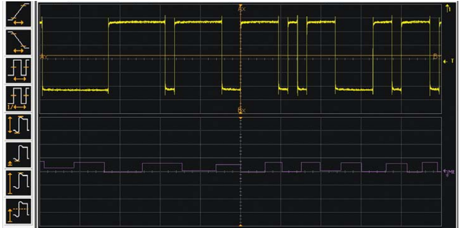
Figure 24. A trend display, showing a time plot of the measurement time-correlated with the signal waveform data, makes it easy to understand relationships between jitter and signal conditions.
