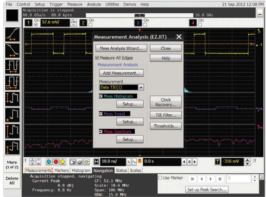
Figure 20. The setup wizard prompts you to select measurement thresholds, histogram, jitter trend, and/or spectrum displays.
