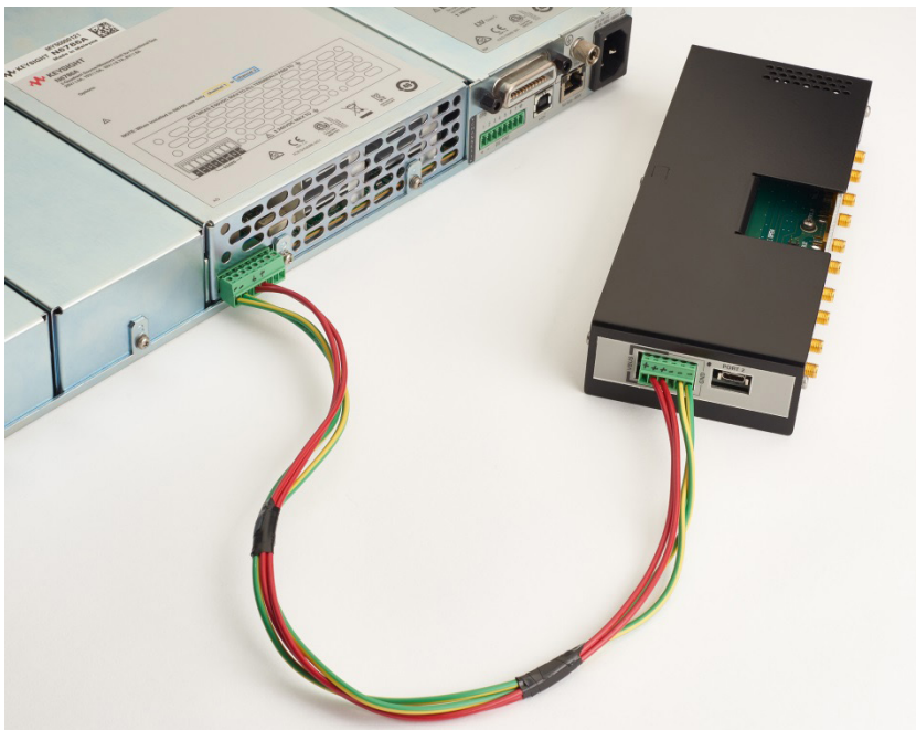
Figure 9. Use an external power supply to supply extended power (up to 5 A, 20 V) to the USB device. A power supply plug connector is included in the N7016A kit.
