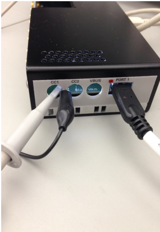
Figure 7. The CC1, CC2 and Vbus signals can be conveniently probed from the N7016A using a Keysight passive probe.
