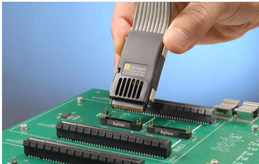
Figure 22 Midbus aligned over back plane
