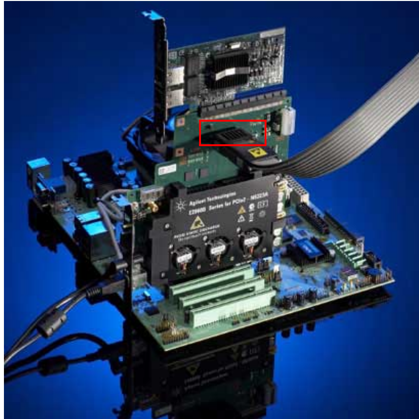
Figure 12 Midbus probe plugged into the retention module
