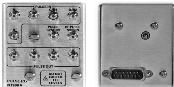
Pulse I/O adapter (N1966A) simplifies connections
