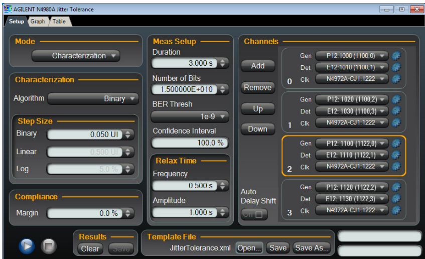
Figure 9. Jitter tolerance setup panel in N4980A
