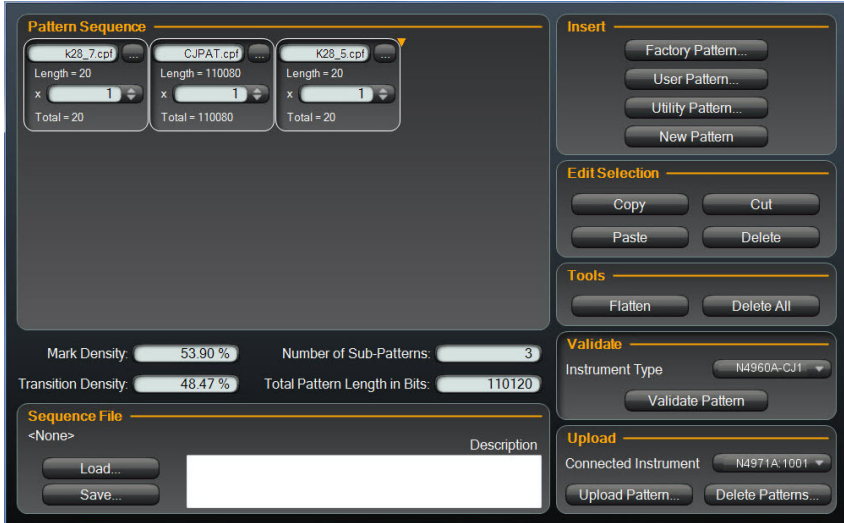
Figure 5. Programmable pattern editor
