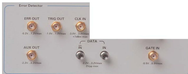
Figure 15: Front panel connectors for error detector.
