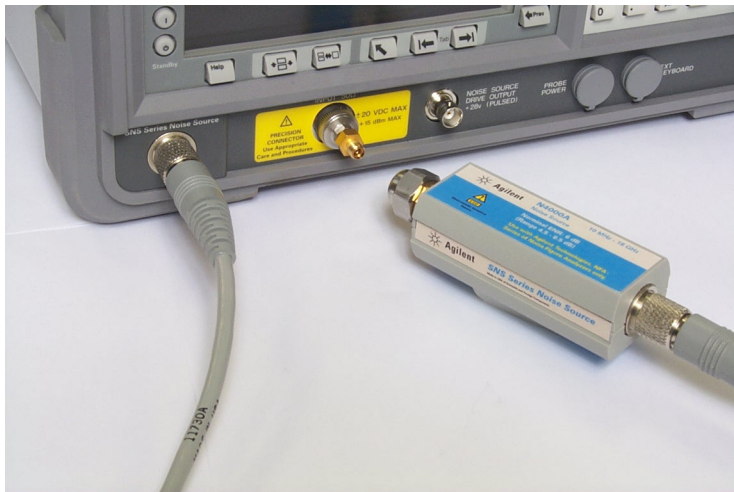
Figure 1-8 Operator's Check Test Setup for T_{\text{cold}} Communication
