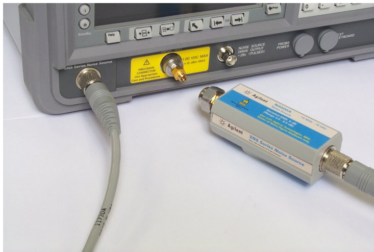
Figure 1-5 Operator's Check Test Setup for Data Communication
