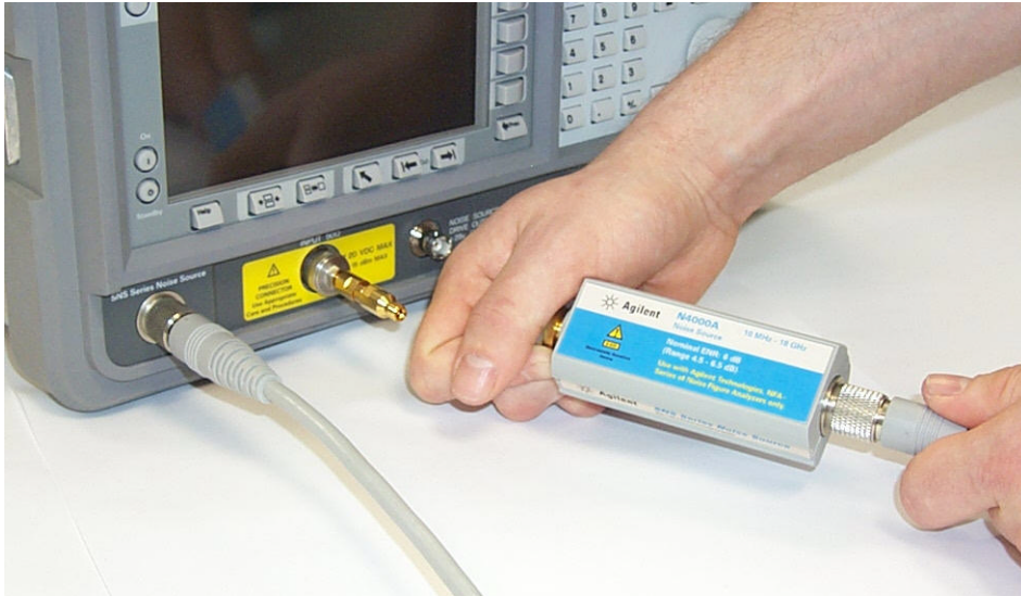
Figure 1-11 Operator's Check for T cold Upload From SNS
