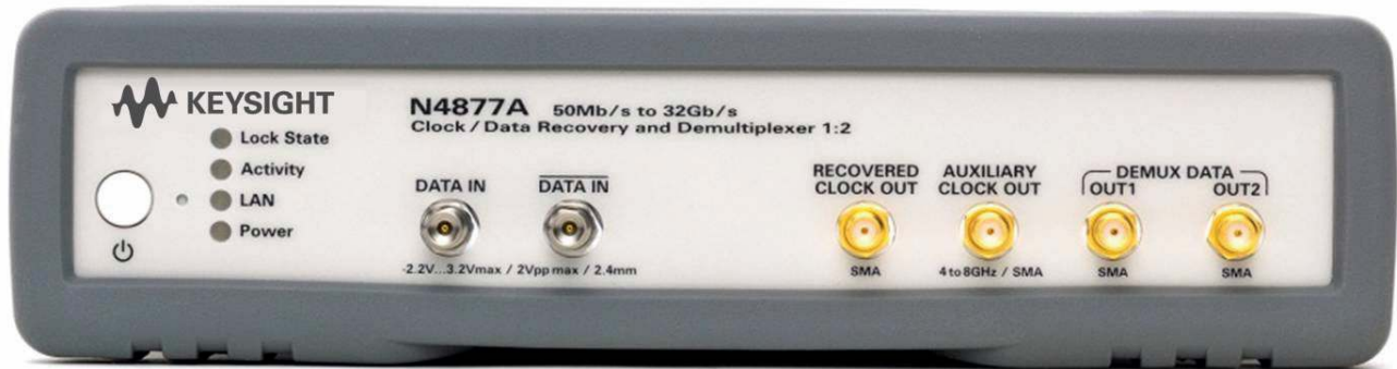
Figure 2. The N4877A recovers clock and demultiplex data from 50 Mb/s to 32 Gb/s
