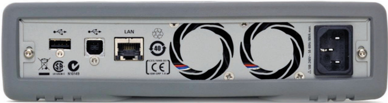
Figure 11. USB and LAN connection are located at the back of the Keysight N4877A clock data recovery and demultiplexer 1:2.
