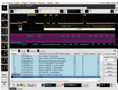
Trigger on and decode MIPI packets
