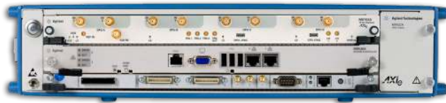
Figure 21. One Agilent M9703A AXIe 12-bit digitizers and one M9536A embedded AXIe controller installed in the Agilent M9502A 2-slot AXIe chassis.
