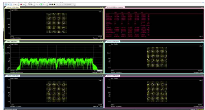
Figure 8. The M9703A-LDC option provides real-time digital downconversion for up to 80 MHz frequency span per channel (160 MHz in I+Q mode), ideal for emerging communications standards research and design validation. Here we show the analysis of four 802.11ac 160 MHz wide baseband signals. The M9703A allows to reach an EVM of down to -45 dB.
