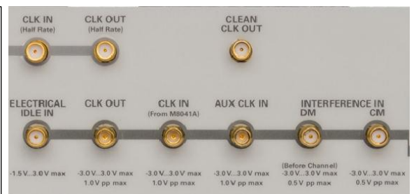
Input connectors for level interference (on the right side)
