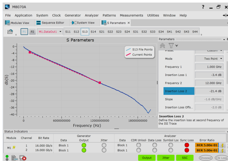
Adjust loss and import of S21 parameters, preliminary M8070A screen shot
