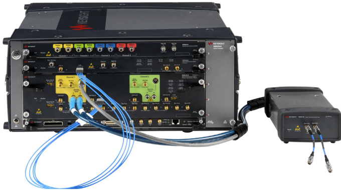
Figure 3. The remote head M8057A is required for each channel and is required for NRZ and PAM4 signals. It contains an adjustable gain amplifier without re-timer. Users can select NRZ or PAM4 coding and de-emphasis taps settings from the user interface with no need to reconnect cables. The cable between the remote head and the module is 0.85 m long. This allows positioning the remote head closely to the test board for the device under test.
