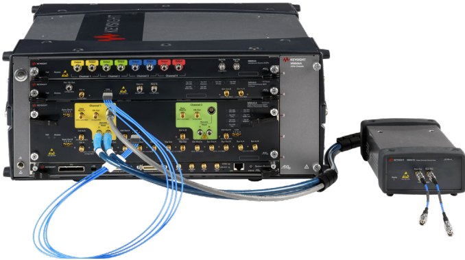
Figure 3. The remote head M8057A/B is required for each channel and is required for NRZ and PAM4 signals. It contains an adjustable gain amplifier without re-timer. Users can select NRZ or PAM4 coding and de-emphasis taps settings from the user interface with no need to reconnect cables. The cable between the remote head and the module is 0.85 m long. This allows positioning the remote head closely to the test board for the device under test.
