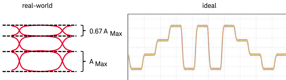
Figure 8. PAM4 eyes can show a level separation mismatch. Receivers must be able to detect the digital signal content properly within the given mismatch ratio.
