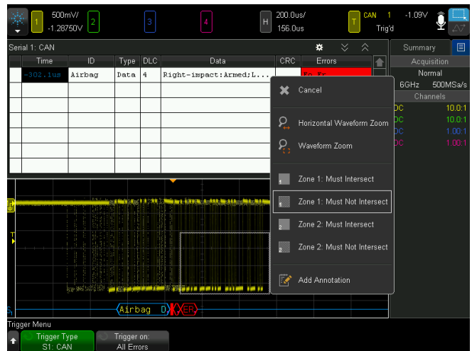
Figure 13. Setting up the InfiniiScan Zone trigger in addition to a CAN bus error packet trigger.
