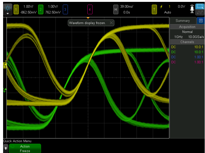
Figure 57. Quick Freeze Display preserves the persistence.
