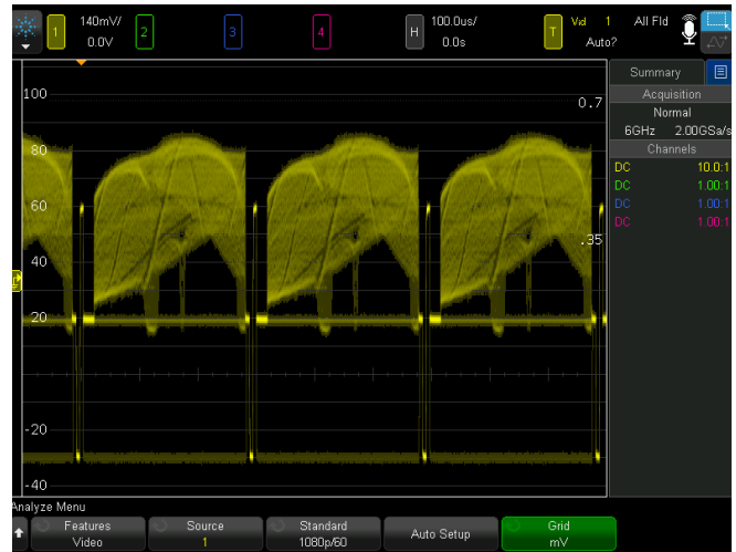
Figure 45. Triggering on a 1080p/60 signal.
