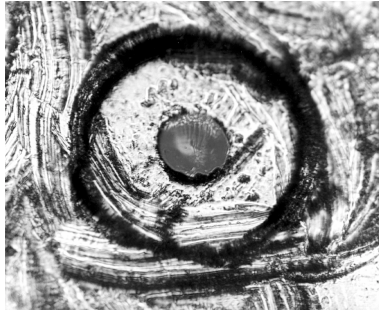
Figure 3-6. Damage from improper cleaning.
