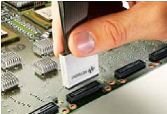
E5385A 34-channel Samtec connector probe
