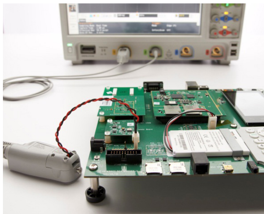
N2820A high-sensitivity 2-channel current probe
