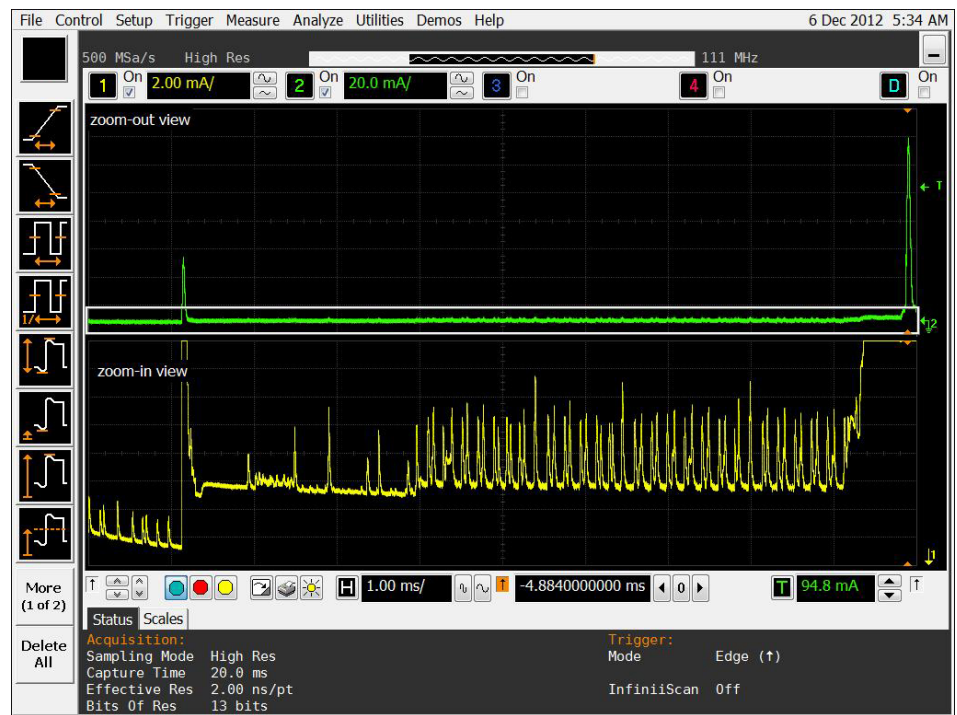
The N2820A 2-channel current probe connects to two oscilloscope channels to provide simultaneous low- and high-gain views for wider dynamic range measurement
