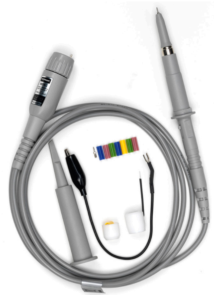
10076C high voltage passive probe
