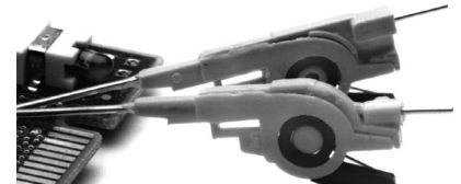
Extremely small-sized clips for probing PQFP and SOIC SMT packages.
