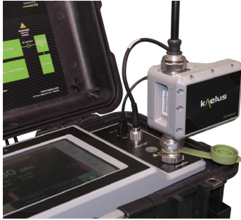
Range to Fault (RTF) Module
