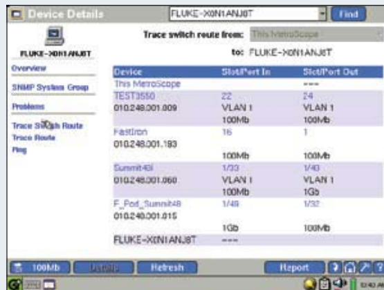
TraceSwitch Route™ shows how devices are interconnected in a switched network.
