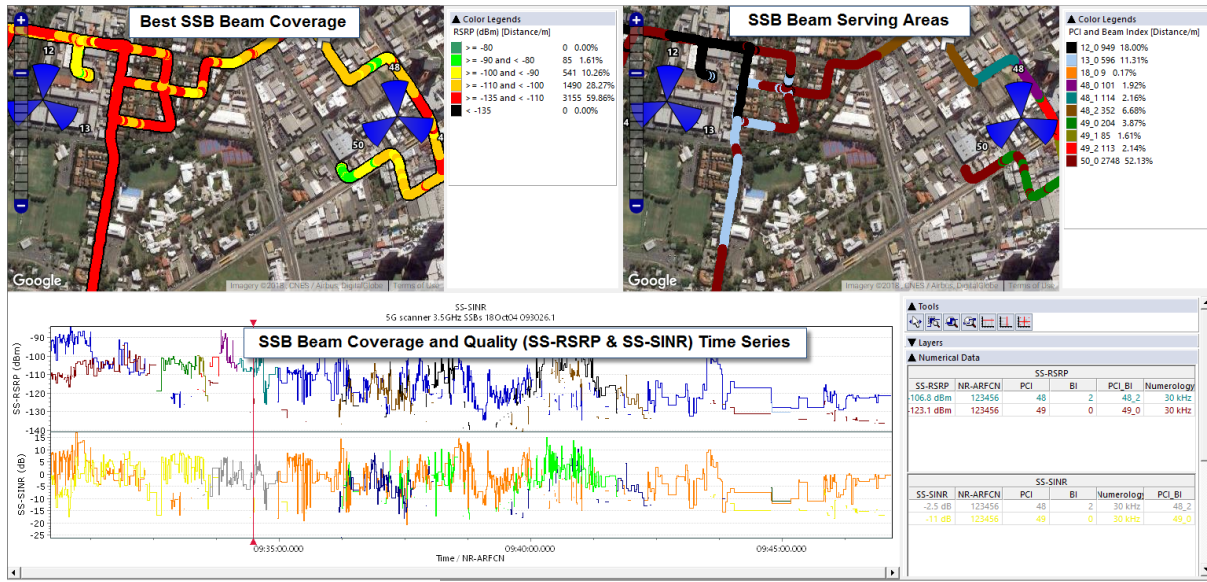
Figure 7. Example of Nemo Outdoor 5G NR scanner measurements. Coverage and quality metrics, namely SS-RSRP, SS-SINR, are reported per each SSB reference beam of a cell.
