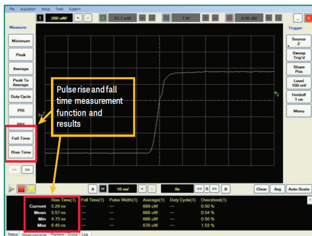
Figure 14. Radar pulse parameters (timing) analysis
