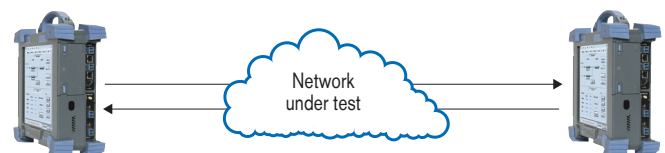
■ Dual-test-set configuration (arrows show direction of traffic).
