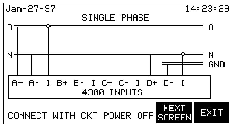
The purpose of this screen is to enable users to verify that all probes have been connected properly. If *not* connected properly, power OFF the PP4300 immediately. Make any necessary changes to the connections, and start the tour over again at 5.3 *Power ON the PP4300*.
