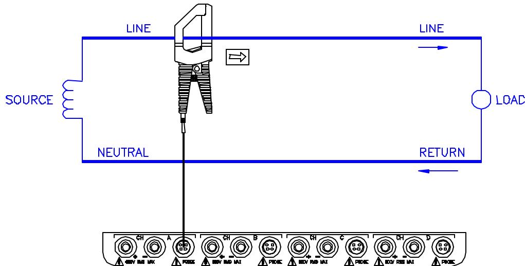
The connection shown above is not recommended without a voltage connection to ensure frequency synchronization. If this configuration is used, then an internal frequency reference must be entered.
