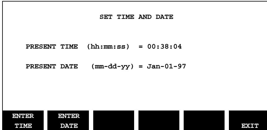
To change the time, press the **ENTER TIME** SOFTKey; Note that the SOFTKey options have changed to facilitate setting the time:
