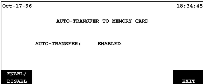
Press the **EXIT** SOFTKey to return to the “Memory Functions” screen.
