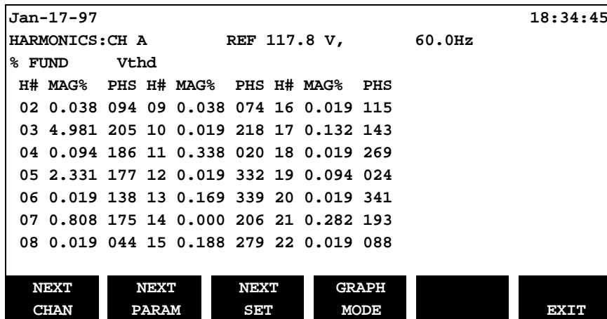
Mag% is the amplitude of the harmonic. PHS is the phase angle between the harmonic and fundamental of the channel displayed.
