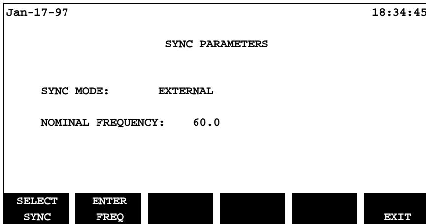
Press the **SELECT SYNC** SOFTKey to toggle through the sync mode options. Press the **ENTER FREQ** SOFTKey to enter the frequency (using the numeric keypad). Exit by pressing the **EXIT** SOFTKey.
