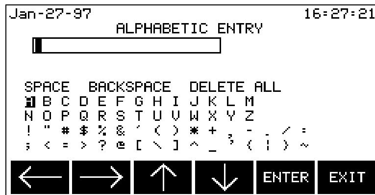
The arrow SOFTKeys are used to highlight desired letters. The **ENTER** SOFTKey moves highlighted letters into the small text window at the top of the display area until the site/file name is completed. Use the numeric keypad for numbers.
