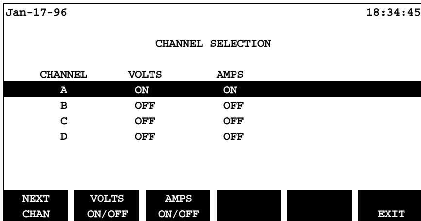
This screen is used to filter data for display on the "Scope Mode" screen. Toggle volts and amps ON or OFF for each channel as desired. Press the **EXIT** SOFTKey to return to the "Scope Mode" screen.
