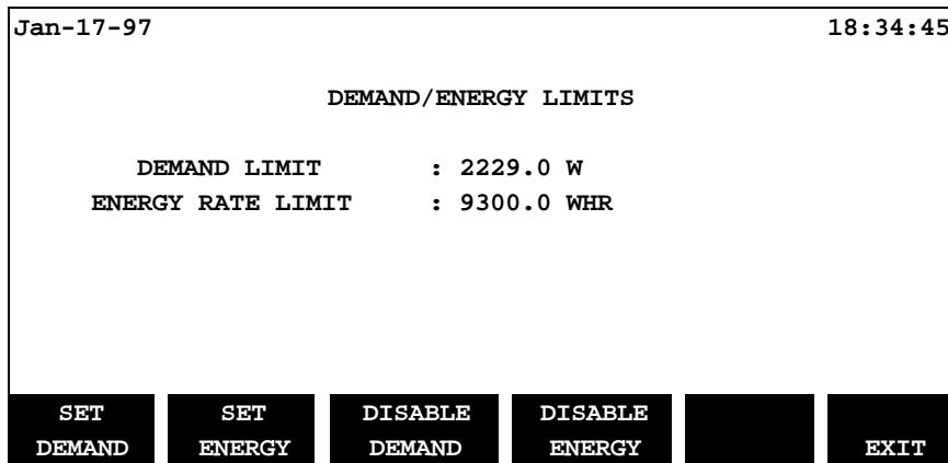
Use the SOFTKeys to **SET**, **ENABLE** or **DISABLE** the limits. The consequences of enabling and setting these limits are as follows:
