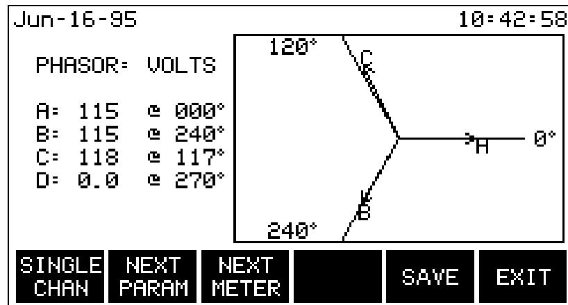
**Correct 3-phase current phasor connections**
