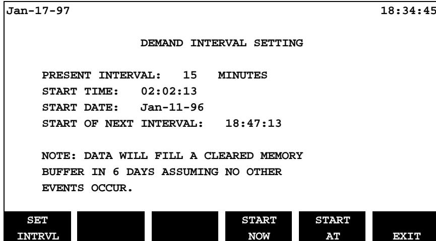
Press the **SET INTRVL** SOFTKey to change the interval start time and date (watch the screen carefully when selecting this – especially the SOFTKeys -- note that ENTER and BACKSPACE SOFTKeys become operational).
