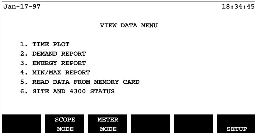
**Step 1** From the “View Data” screen, press the **1** key to display the first of the Time Plot graphs.
