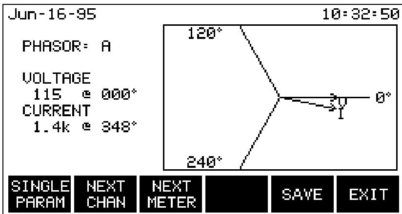
**NOTE** - All phasor diagrams for connections E.4 through E.10 (on the following pages) are drawn assuming balanced, resistive loads.
