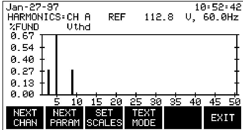
**Step 2** Explore some options -- press the **NEXT CHAN** SOFTKey to advance through the channels. Press the **NEXT PARAM** SOFTKey to change parameters (by highlighting and selecting the desired parameter from a list).
