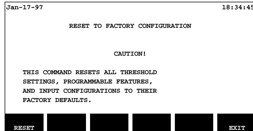
Press the **EXIT** SOFTKey to return to the “Memory Functions” screen (without actually resetting to factory configuration).
