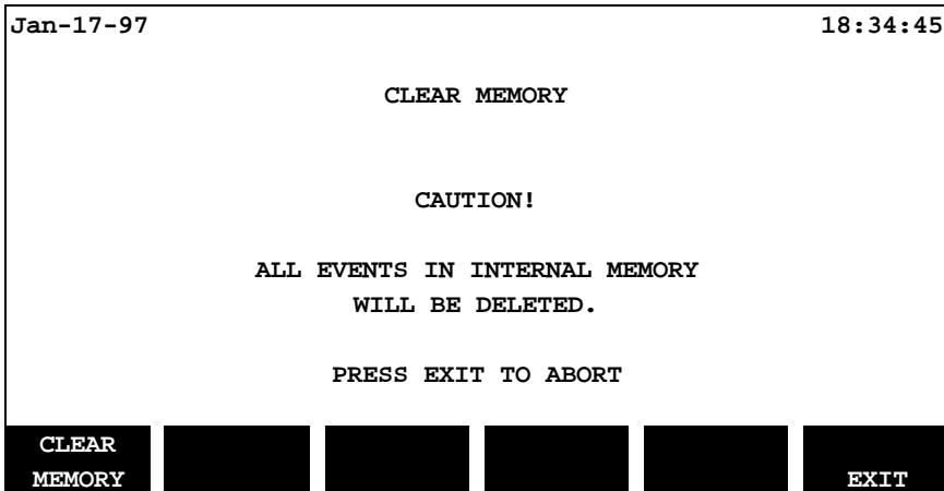
Press the **EXIT** SOFTKey to return to the “Memory Functions” screen without actually clearing any memory.
