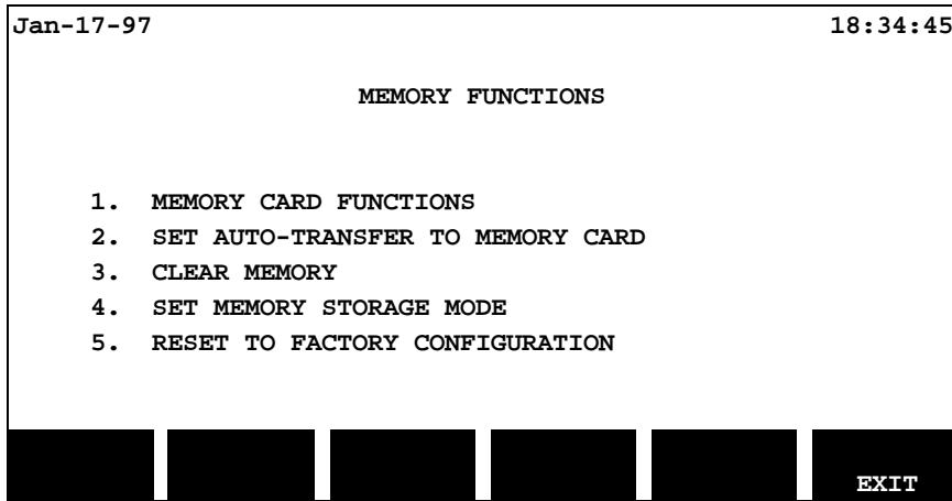
**Step 6** Press the **1** key on the numeric keypad to display the **Memory Card Functions** screen. This screen displays the status of the memory card installed. Use this screen to read and write event and setup data on the memory card and to format the memory card (see Appendix F).
