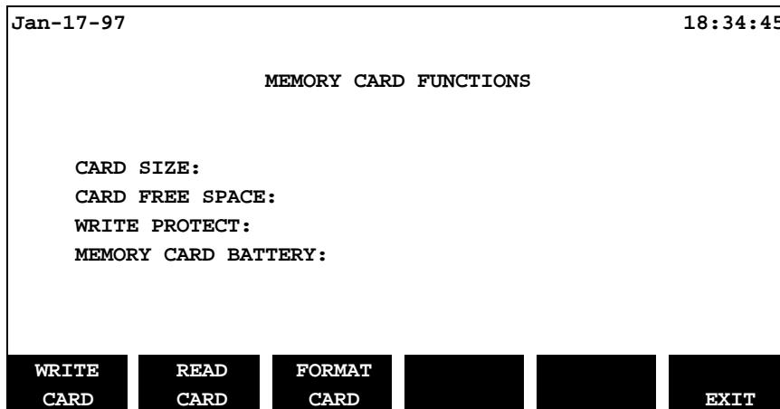
**NOTE** - If the memory card is not formatted (or not seated in the slot properly), no values will be displayed. New memory cards are not formatted and must be formatted before use.
